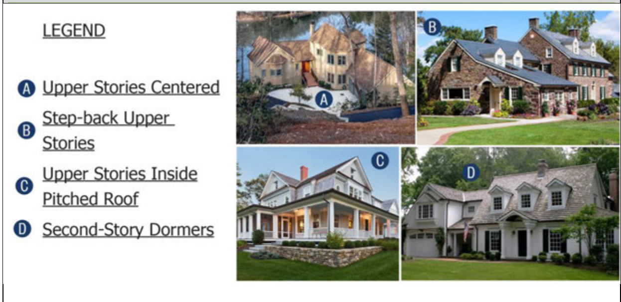
FIGURE 7.1.4:D:5: BUILDING FORM
