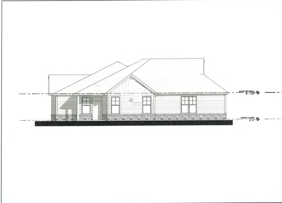
BUILDING 2 - LEFT ELEVATION 4 3/8" = 1'-0"
