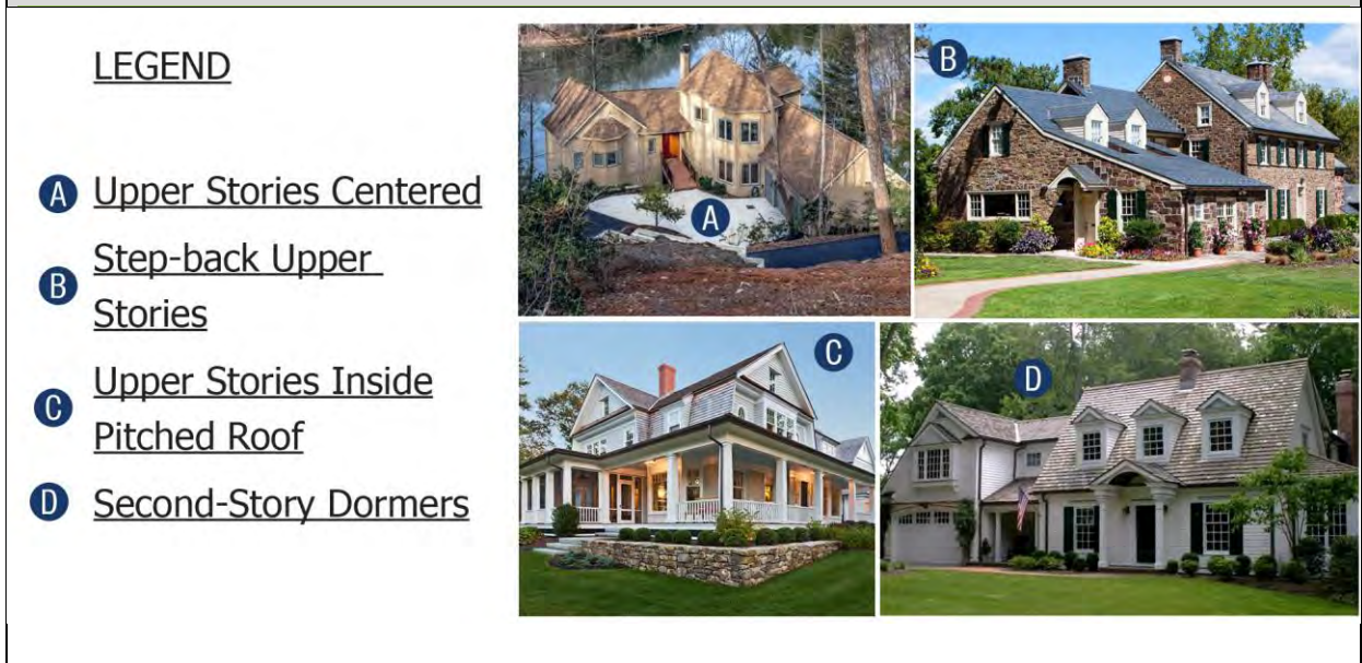
FIGURE 7.1.4:D:5: BUILDING FORM
