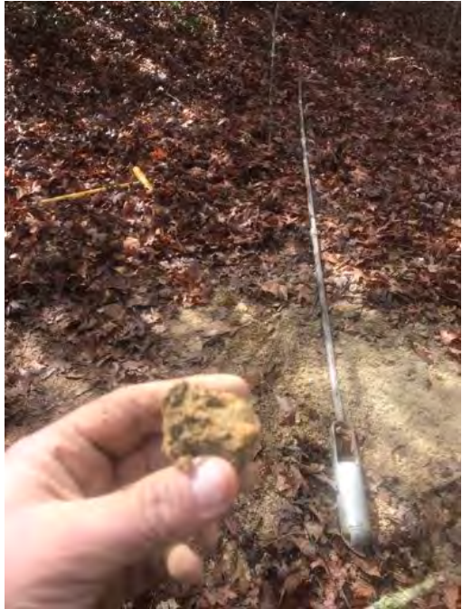
Image 6- Tools (extendable hand auger and utility probe) used to excavate soils for borehole characterization.
